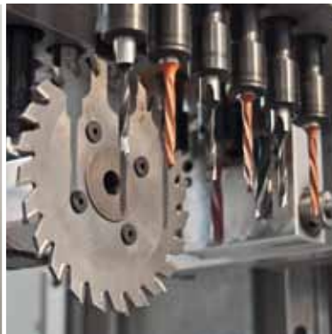
Drilling unit with horizontal-vertical spindles and grooving saw Ø120 mm
