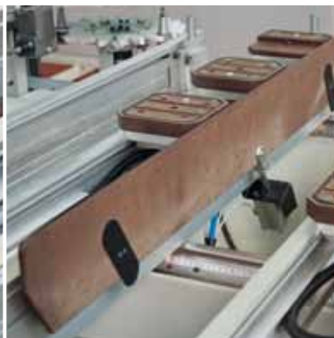
Feeding bar supports
