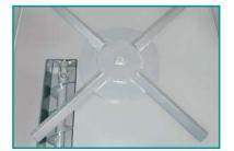
The continually turning tube extractor mixes the material and sends it to the discharge screw conveyor, which feeds it cyclically to the pressing mechanism.
