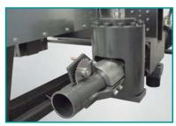
With the automatic briquette length feature the length of the briquettes can be constantly maintained even with a variety of materials.
