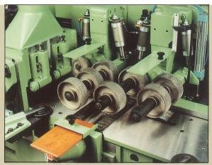
Infeed Features: Infeed driven pneumatically linked bed roller. Dual, independent top head chipbreaker shoes. Roller side pressures. Multiroller infeed drive.
