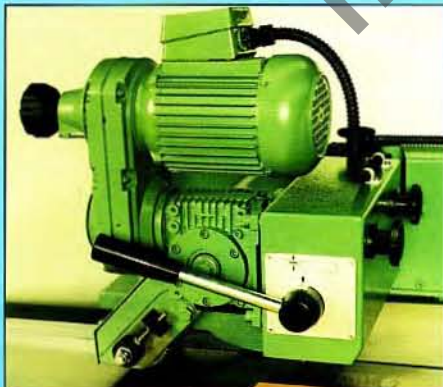
Patented swinging arm power feed unit
