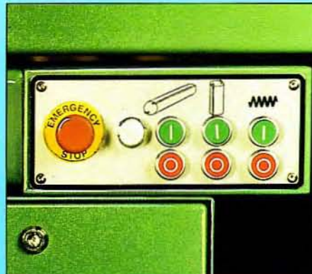
Operator controls readily at hand with master stop at both infeed stations.
