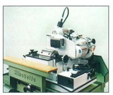
By simply turning the head arrangement through 90 degrees a change over can easily be made from profile to straight knife grinding.
