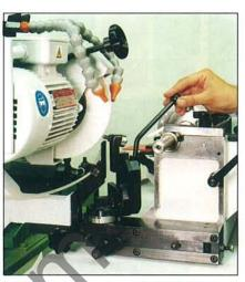
Safety is ensured with the unique diamond dresser design which keeps the operator clear of the wheel.
