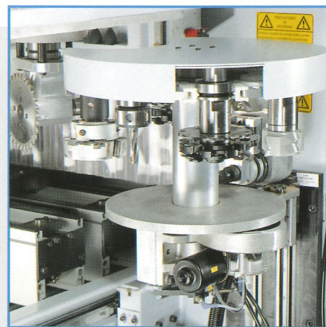
BP150 with 8-fold change plate magazine
