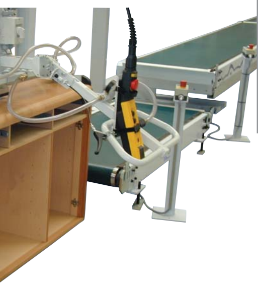
Final assembly with vacuum lifter MTB 100
