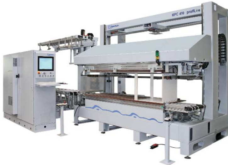
MPC 410 – automatic jointing clamp
