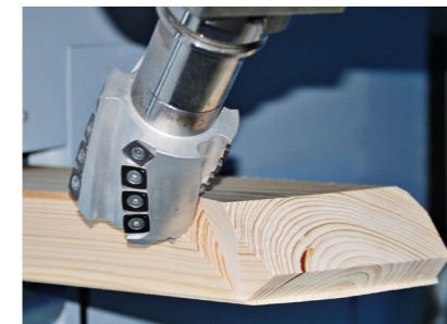
Producing a tenon joint
