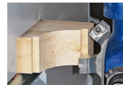
Machining the rafter head
