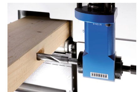
Production of mortises and pockets
