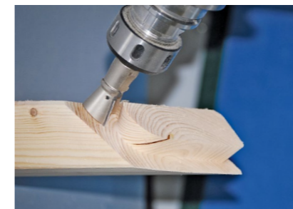
Dovetail at the jack rafter
