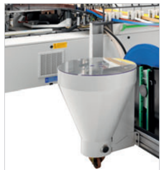
Multiple reel magazines available from 2 to 24 positions. Glue tank feeder from ground.
