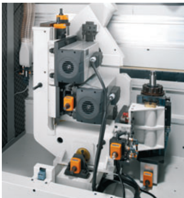
Compact antisplint+double hogger unit.
