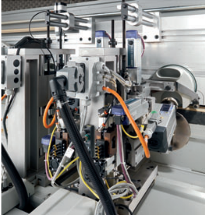
RF40 - Multiprofile fine trimming unit.
