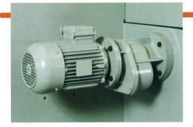
Feeding track is powered by a geared motor controlled by an inverter.
