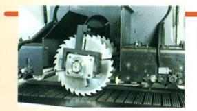
The surface treatment of the spindle ensures perfect running of the moving blade and long working life.
