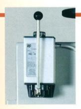
Machine lubrication is by a manual pump.
