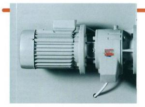
Feeding track is powered by a geared motor with 2 fixed speeds: 12 and 24 m/min, which can be selected via a selector switch on the control panel.
