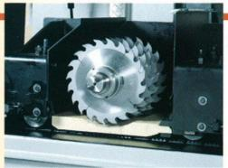
The blades are mounted directly on the spindle (blade sleeve optional).
