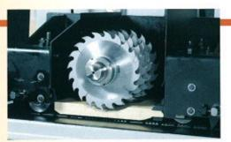
The blades are mounted directly on the spindle (sleeve optional).
