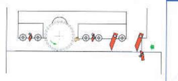
TOP ROLLERS GROUP raised automatically, with 5 independent hold-down rollers and a long wooden shoe placed between the blades.
