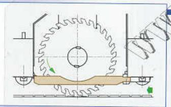
The long wooden shoe allows perfect holding of the plank, even if warped in the blade compartment, thus preventing the blades from removing or splitting cracked or thin planks.
