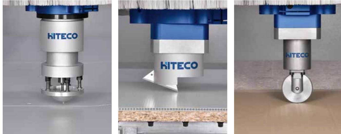
A range of dedicated heads for the machining of advanced materials, such as plexiglas, plastics, alucobond, aluminium, polyurethane forams and honeycomb cardboard.
