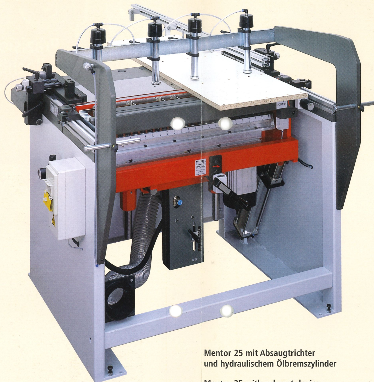
Mentor 25 with exhaust device and hydraulic oil brake cylinder
