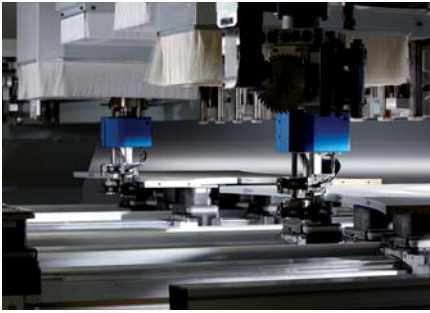
Finish processing of furniture component edges
