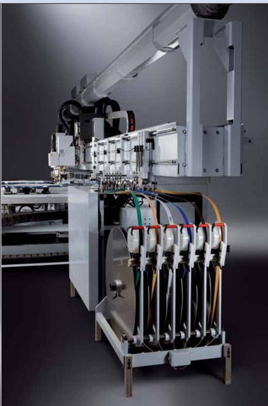
Edging magazine with coupled motion in the X direction with up to 6 coils or externally with up to 24 coils
