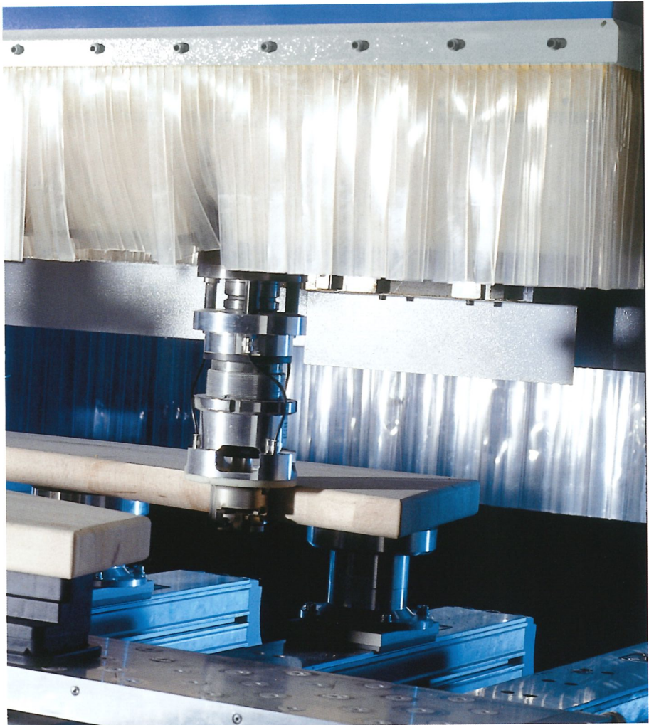
Scraper blade processing with the traced combination flush trimming and scraping unit
