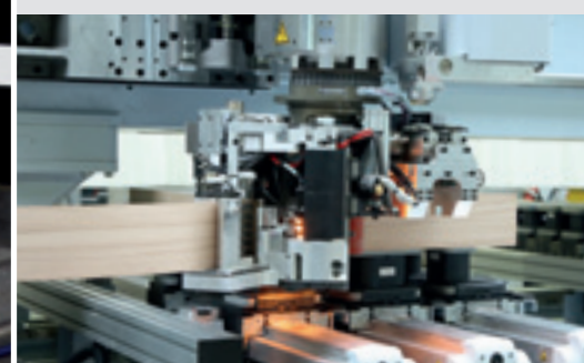
Edge banding for components up to 100mm in height
