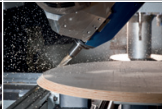
Chamfer trimming on a table top
