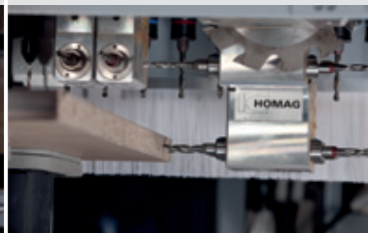
Horizontal boreholes for carcass connections
