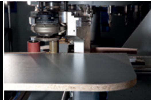
Gluing unit easyEdge for efficient banding onto shaped components
