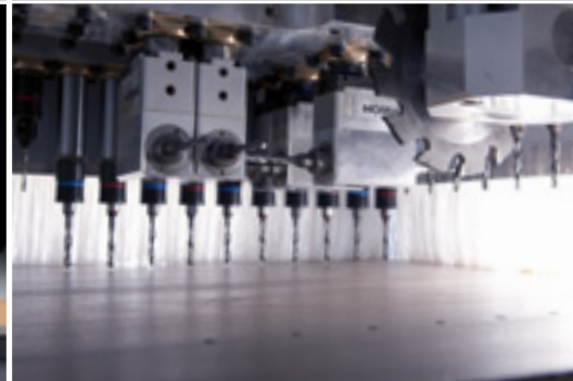
High-speed drilling technology with grooving saw
