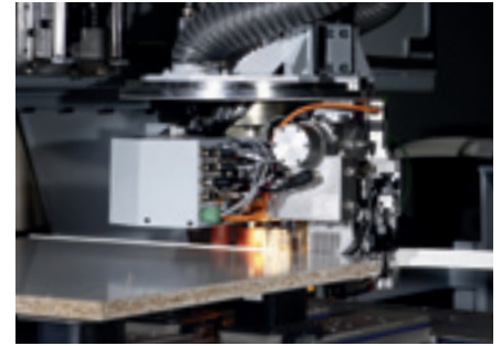
Edge banding to a previously unattainable standard of quality: HOMAG laserTec – the quantum leap for furniture production.
