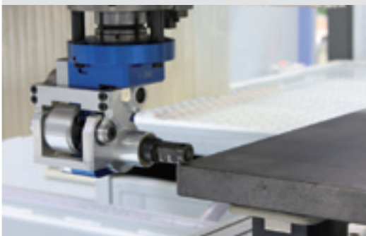
Traced flush trimming of overhanging edges on postforming profiles
