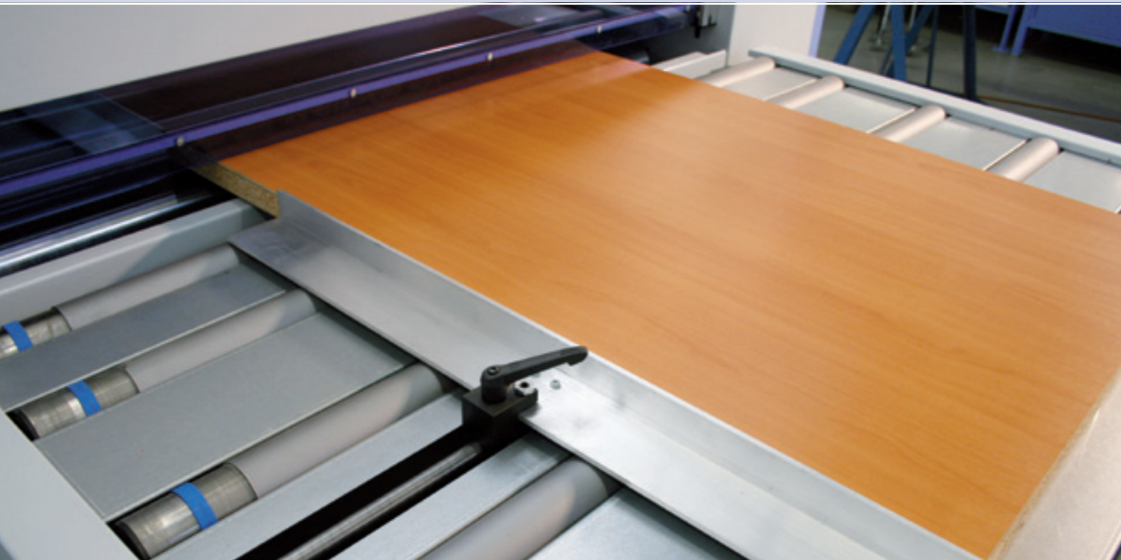
Fence guide for accurate positioning of the workpieces on the machine for an exact processing result
