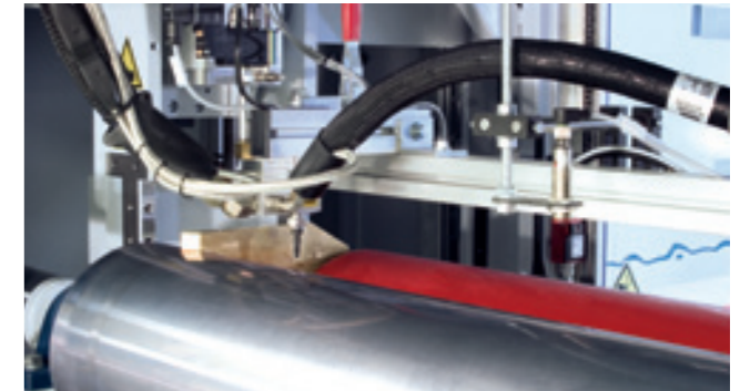
Regulation and application roller with special sealing system for an efficient and clean production
