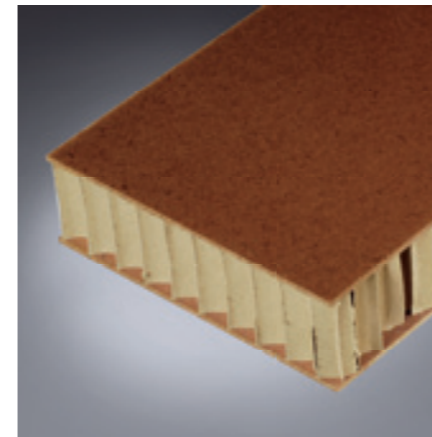
Paper honeycomb with MDF layer
