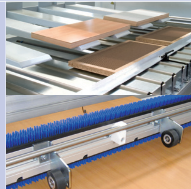
Top picture: Motorized positioning rack for material storage and simplified positioning of workpieces
