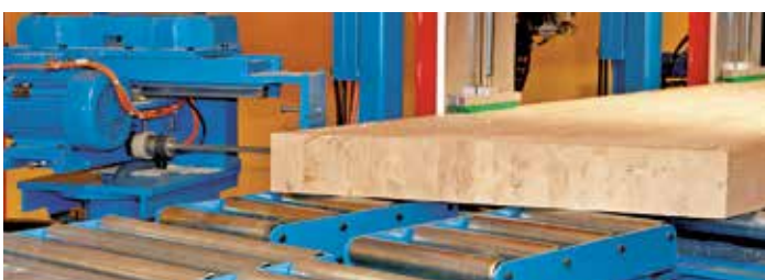
360° pivoting deep-hole drill unit up to 1250 mm
