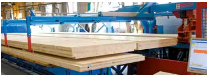
Automatic infeed system also for glulam panels
