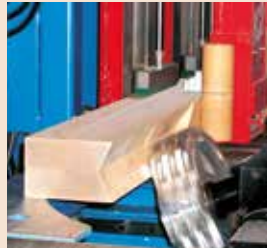
Channelling or hip ridge cuts without rest wood
