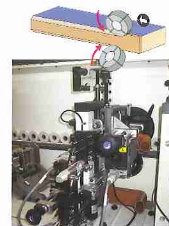
Bündigfräs-/Fasaggregat Fine trimming unit
