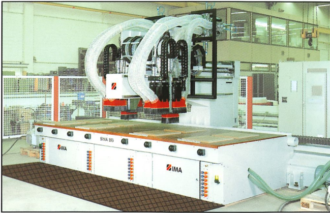
BIMA 610 with continuous worktable and 2 main spindles for split panel loading.
