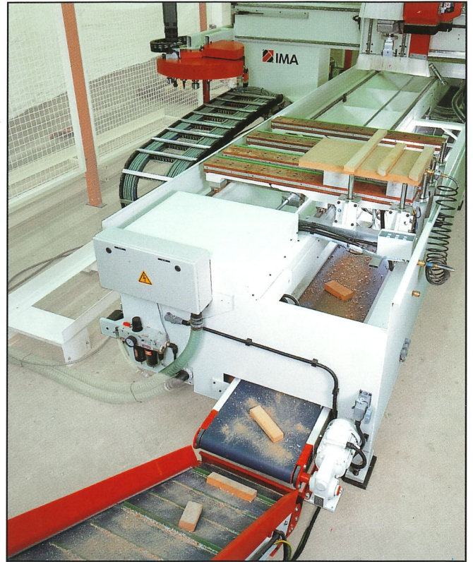
Optionally, the BIMA 610 may be equipped with a chip transport band. Chips and residuals will be removed automatically and will therefore impair neither the feeding nor the processing.
