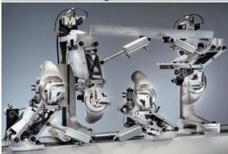
Schwenkarmkopier-Aggregat (SKF) Contour trimming unit
