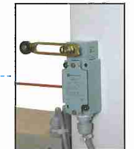
Finecorsa apertura piano Limit switch for press opening Endscharter "Öffnung Presse"
