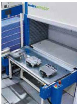
The full tray extraction device was designed to improve the handling of heavy and bulky goods, an operation which requires the aid of a lifting device. With the full tray extraction device, a tray is placed in front of the access opening for loading and unloading purposes. This can be loaded onto the optional transport cart for safe and easy handling.
