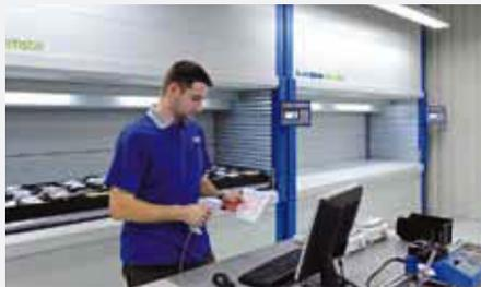
Fast and easy integration of barcode scanners for order identification, picking and confirmation.
