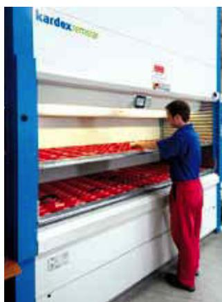
Thanks to the double-access handling option it is possible to use two work levels in the access opening. A tray is transported into the first work level in the access opening and the shutter door closed. While articles are stored or removed, the next tray is being retrieved and kept in a waiting position behind the access opening.
