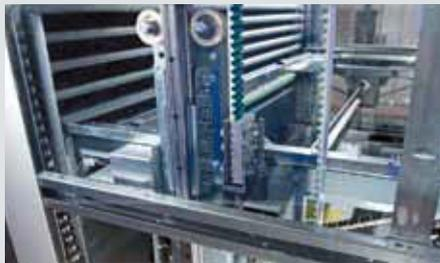
The extractor device delivers the requested tray to the access opening or back to a free storage location within the device at fast speeds. At the push of a button or scan of a barcode.
