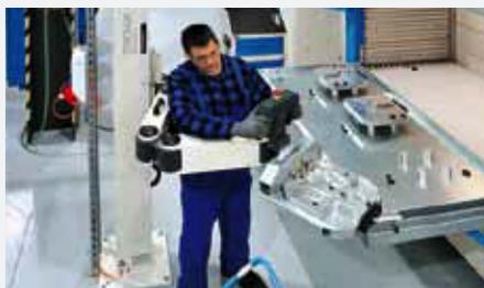
Easy integration of hoists, cranes, grippers and manipulators for additional ergonomic material handling.
