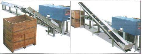
Disposal of waste can alternatively be right-angled or in parallel to the entry table respectively the exit table (Option C).
