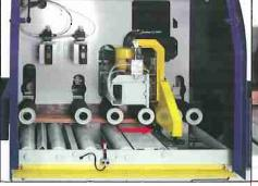
The cutting speed is adjustable steplessly (cutting time < 0.1 sec). During the cut downholders safely fix the work pieces.
