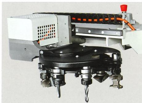
It is possible to have the machine fitted with **Rapid 8**, a supplementary tool magazine anchored to the mobile gantry, for an even faster tool change-over.
