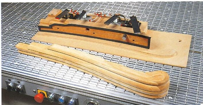
Inverted "T"-shaped grooves and a series of threaded holes provide perfect fixing for all holding-down devices.
