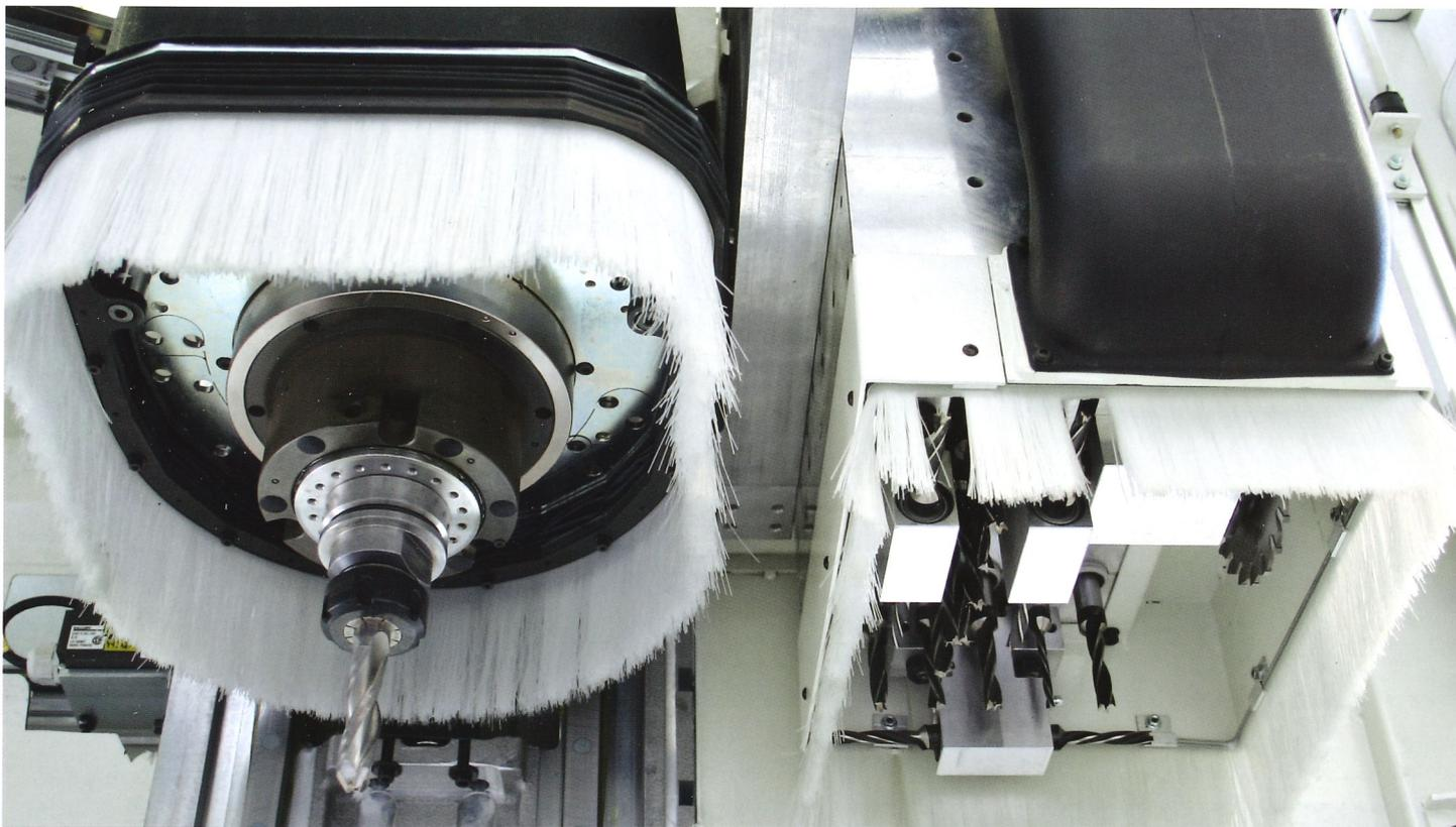
The machining head consists of an 8.5 kW routing unit. It can accommodate a boring unit with 7 vertical spindles or 18 spindles (12+6) with integrated sawblade.
