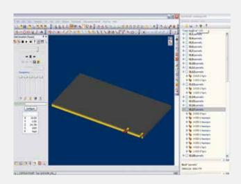
Maestro Beam&Wall, developed from the experience of SCM, allows to interface with the industry's best design CADs available on the market. With a few clicks, it is possible to switch from importing BTL files to running the work piece in the machine. It is not necessary to program the single elements, because Maestro Beam&Wall gets all the information from the CAD that designed the structure, and the software will do the rest.
