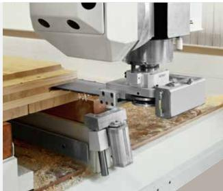
The aggregate "chainsaw" allows to quickly realize:  $90^{\circ}$  openings, cutting with nesting technology, deep grooves and slots on all sides of the element.
