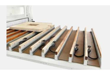
The **flexible worktable** is equipped with a number of options allowing to refer and block elements of different shapes and sizes.
