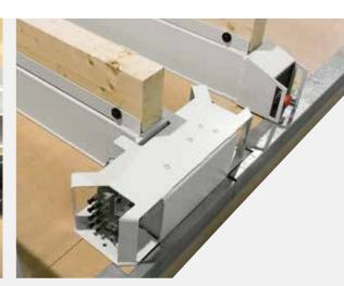
Even small work pieces can be blocked on the worktable thanks to the suction cup system. The suction cups with automatic exclusion are easily positioned across the work area and connected to the vacuum ports arranged on the machine with quick plug-in connectors on the perimeter of the table.
