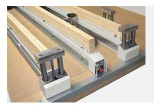
Heavy duty reference system on the sides of the worktable, to properly accommodate panels with large dimensions. After the work piece positioning, the reference stops are automatically lowering, leaving all the sides of the piece free for further processing.
