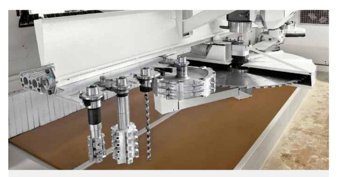
Dedicated positions for special aggregates: **sawblade with up to 1020 mm diameter**, chainsaw and planing aggregate.
