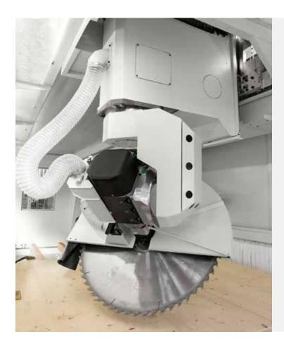
Machining head unit and electrospindle are specially designed to perform all the operations required for the production of construction elements with heavy duty stock removal.
