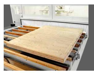
The positioning of bulky and heavy elements such as CLT/X-lam panels might be awkward and difficult; the **laser system** simplifies this operation projecting the tool paths on the work piece with precision, and allowing the operator to center the program on the piece already loaded on the machine.
