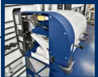
Saw carriage with independent motors for main blade and scoring blade
