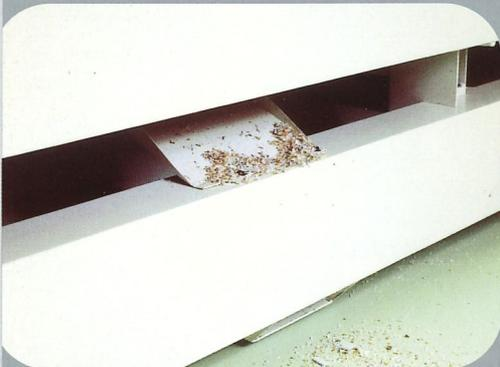
Shavings are removed automatically ensuring that the trimmer's working area is kept constantly clear
