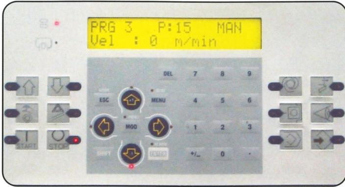
**PLC** control unit with alphanumeric display to avoid micro switch control for the working heads. Enables programming data of each working head, diagnostic function and daily machine production report.
