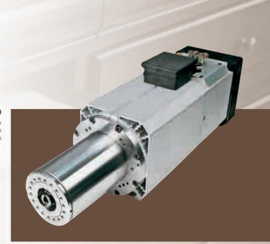
Electro-spindle with constant motor power (S6) 6,6 kW. Automatic tool change with HSK63F tool taper and preset for heads attachment.
