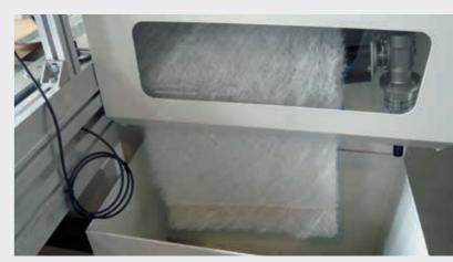
As an alternative, the machine can be supplied with the filtering system FILTER ON DEMAND. A synthetic filtering material is automatically unrolled over the side filtering areas.
