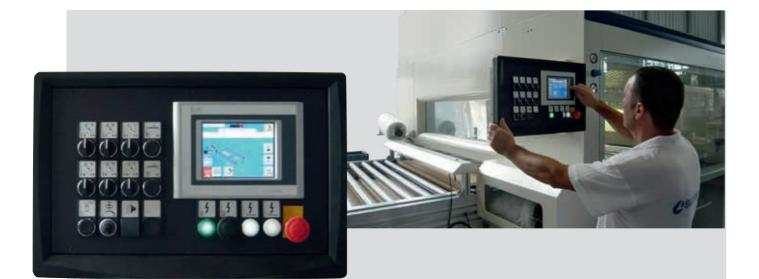
Electronic control via PLC and touch panel; user-friendly software controls the spraying parameters, stores the working recipes, eases diagnostics and programs the ordinary maintenance.
