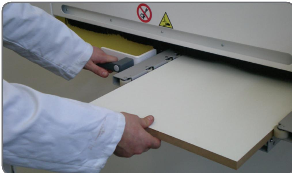
Easy, fast and accurate pneumatic side pusher.
