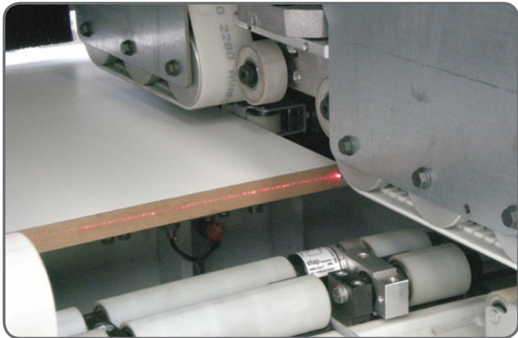
Double "zero" panel reference: one mechanical stop for panel reference in (origin) and one laser photocell (controller by CN) to read the end panel to create a double zero reference. Point 2 automatically corrects the dimension errors of the "X" working position for a perfect coupling of vertical and horizontal pieces.
