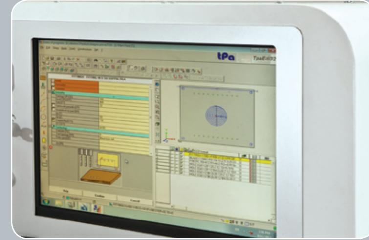
Point 2, Point 3 and Bridge are controlled and managed by a PC : the modern software interface makes particularly easy and direct the machine programming.
