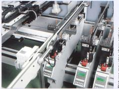
Swivelling drilling block
