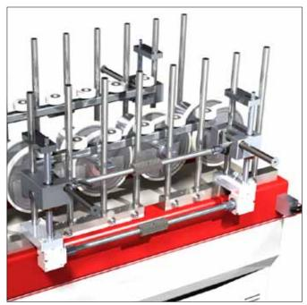
IR LAMP Infrared lamp for profile heating.
