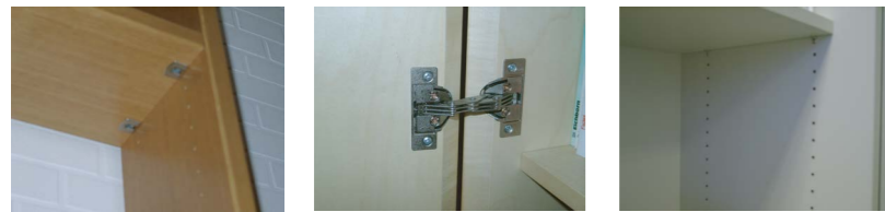
Horizontal Drilling Drilling & Routing Vertical Drilling
