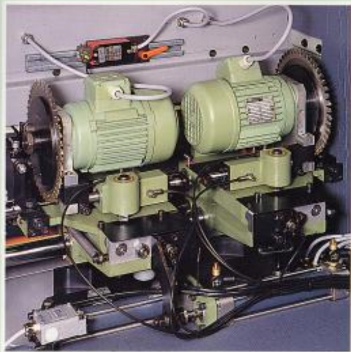
End trimming unit with nr. 2 motors 0,55 Kw, 50 Hz, 3000 rpm, tiltable from 0 to 8 deg., complete with nr. 2 H.M. blades 195x4x80, Z = 48.
