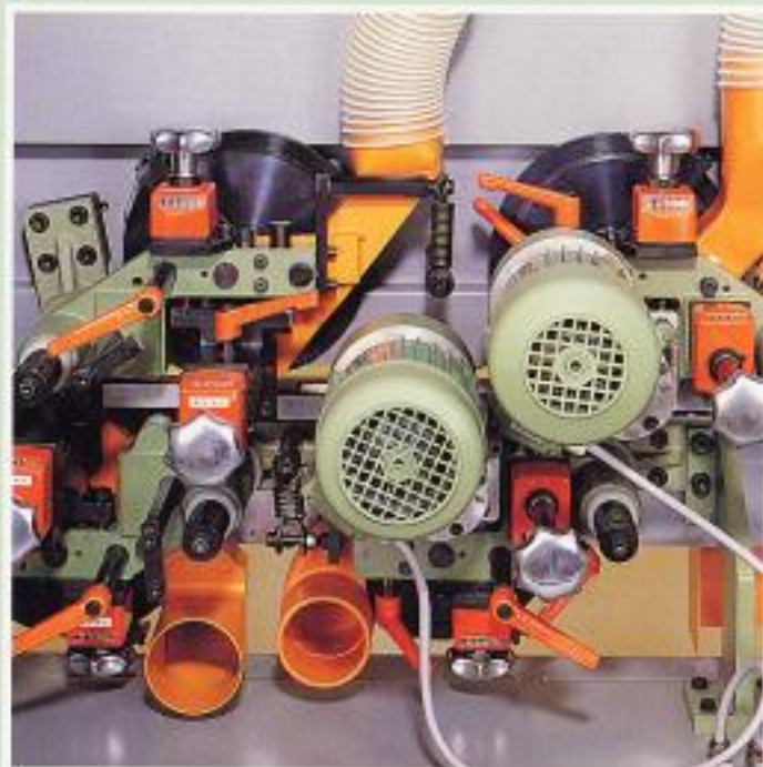
Nr. 1 top and bottom milling/radius/chamfering unit with nr. 2 motors 0,55 Kw, 50 Hz, 12000 rpm; nr. 1 profile scraper unit with vertical and horizontal tracing units.
