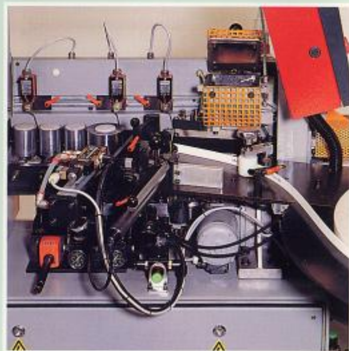
Edge material feeding, gluing and pressure zone.
