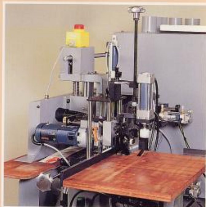
Stationary contour trimmer, range-mounted at end of machine; nr. 1 motor 0,5 Kw, 220 V, 50 Hz, 27000 rpm.
