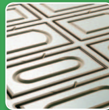
Nesting of cabinet doors
