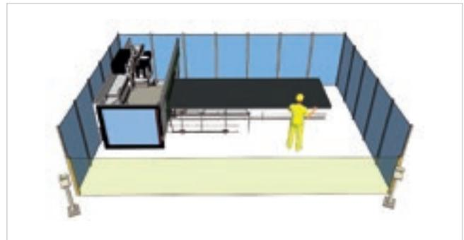
The machine can be configured with tandem loading in order to alternately process panels. This allows for loading or unloading to be carried out during machining operations.
