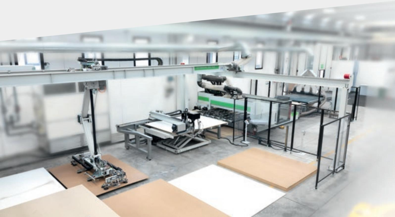
**Winstore** is an automated storage for the optimised management of panels. It ensures that the panels to be machined are easily accessible at all times, so it is possible to substantially increase cell productivity compared to manual loading methods using a forklift truck, without frequent stack changes.
