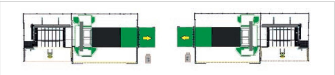
Loading/unloading operations are carried out simultaneously, allowing the operator to remove completed components from the unloading station in the utmost safety whilst the machine is already processing the next panel.
