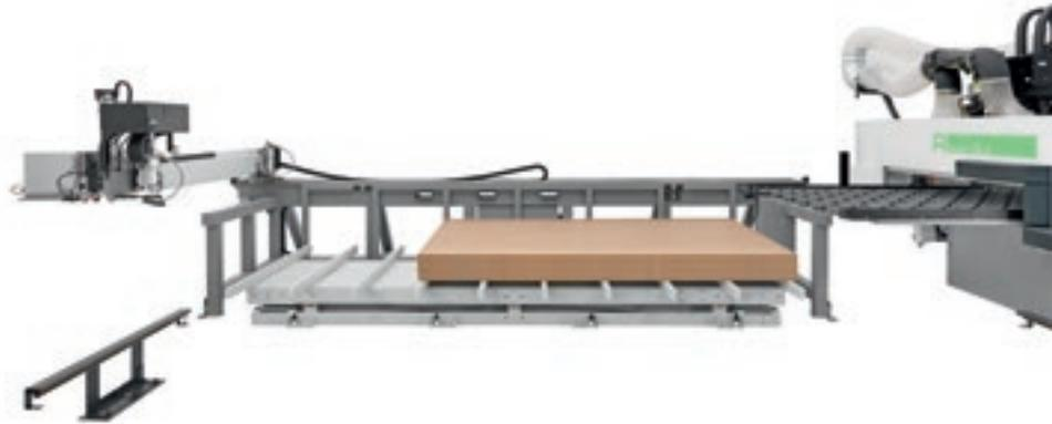
**Panel loading system with scissor lift and automatic panel alignment.**
