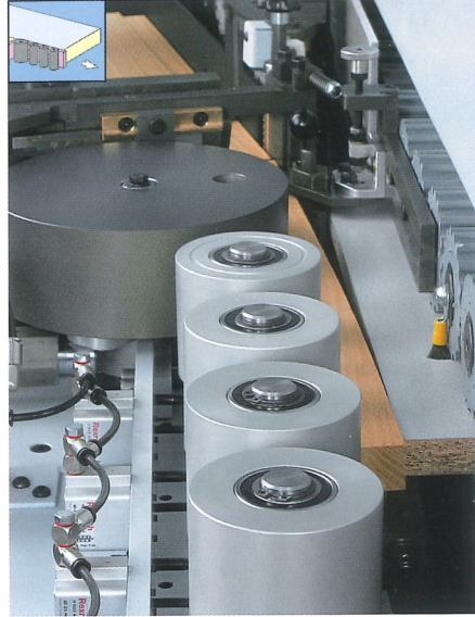
Pressure zone Heavy pressure zone (up to 20 mm) to ensure an optimum glue joint quality.
