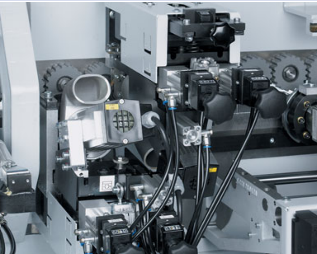
Trimming unit with pneumatic 3-point adjustment
