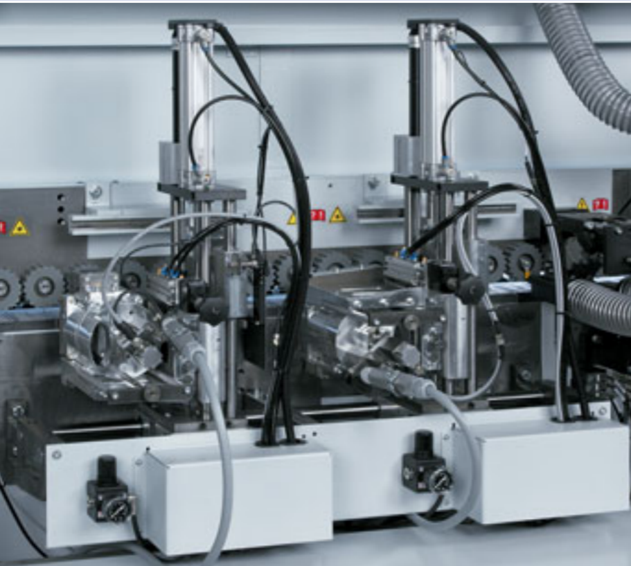
Multifunctional trimming unit MF 50 Trimming of the edge overhang on top and bottom side as well as contour trimming on the front and rear edges. Equipped with an automatic adjustment to switch between thick and thin edges. Workpiece thickness up to 60 mm.
