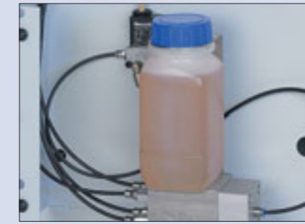
Central lubrication unit
