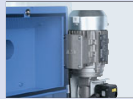
Pressure beam adjustment with servo motor
