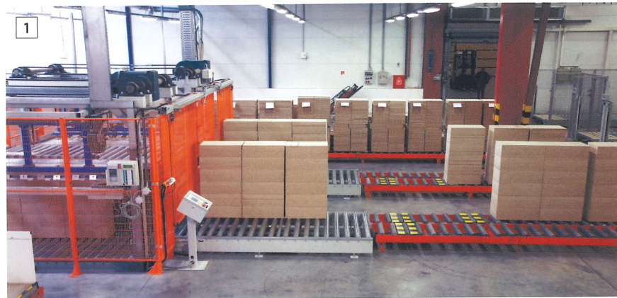
1 Plattenbeschickungsanlage Board feeding device
