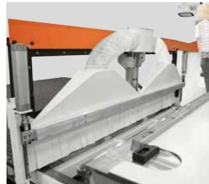
Unloading device with integrated suction system (optional)
