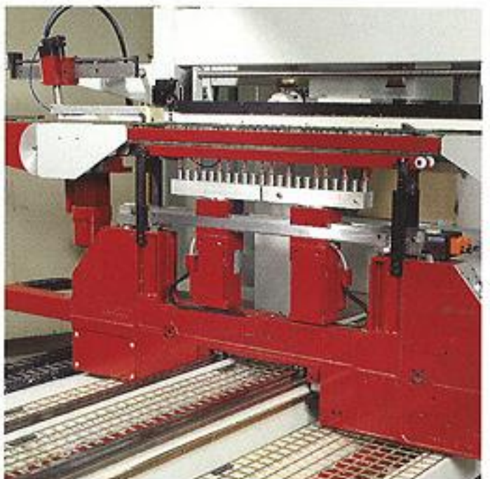
Lower vertical unit clearance, with drill bits mounted underneath the movable horizontal drilling head.
