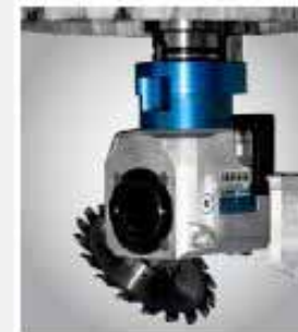
Turn your CNC working center into a 4/5 axis machine thanks to "Disk", a saw/router unit with NC-controlled variable inclination.
