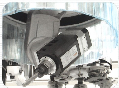
Testata a forare TFR27 con lama integrata TFR27 boring head with integrated saw Cabezal de taladro TF27 con sierra integrada
