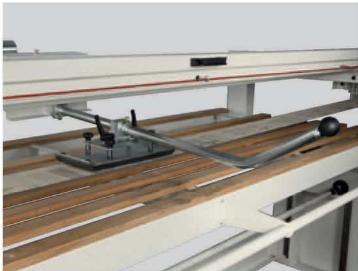
Adjustable pad "Easy Sand" to sand flat workpieces
