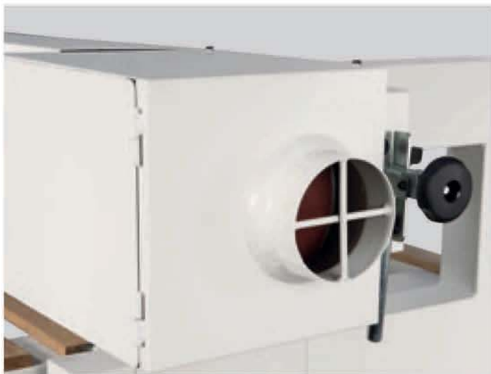
Very efficient dust extraction system with double suction hood on both sides of the sanding belt to obtain best dust extraction results.
