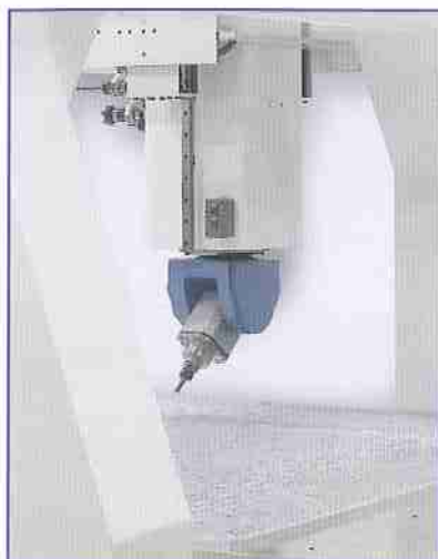
Slitta asse Z a canocchiale per corse superiori a 1000 mm. "Z" axis single shaft electrospindle for strokes over 1000 mm.
