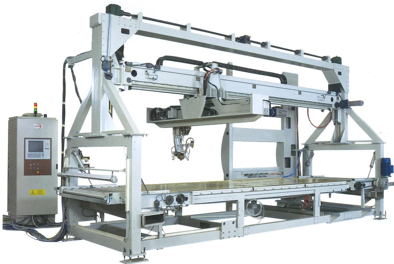
The motion speed of the controlled X- and Y-axes (up to 150 m/min) is reached thanks to special slideways that have a service life of more than 10,000 operational hours.
