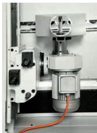
Multiplier device for machining head units
