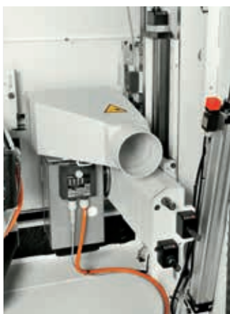
Machining head unit for planing/profiling tools
