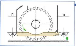
When the machine is used for mult-ripping, the long wooden shoe allows perfect holding of the plank, even if warped in the blade compartment, thus preventing the blades from removing or splitting cracked or thin planks.
