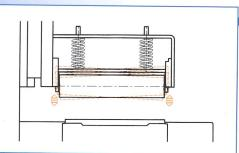
The rollers are guided at the side and they exert pressure over the entire width of the plank through two springs. This application also guarantees good holding of the planks which become curved after drying.
