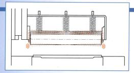
The rollers are guided at the side and they exert pressure over the entire width of the plank through three springs. This application also guarantees good holding of the planks which become curved after drying.
