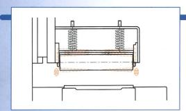
The rollers are guided at the side and they exert pressure over the entire width of the plank through two springs. This application also guarantees good holding of the planks which become curved after drying.
