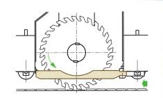
When the machine is used for multi-ripping, the long woodem shoe allows perfect holding of the plank, even if warped in the blade compartment, thus preventing the blades from removing or splitting cracked or thin planks.
