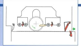
TOP ROLLERS GROUP raised automatically, with 4 independent hold-down rolls and a long wooden shoe placed between the blades.
