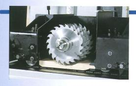
The blades are mounted directly on the spindle. (sleeve optional).
