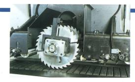
The surface treatment of the spindle ensures perfect running of the moving blade and long working life.
