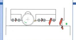
TOP ROLLERS GROUP raised automatically, with 5 independent hold-down rolls and a long wooden shoe placed between the blades. The splinterproof system consists of steel fingers distributed on 4 top rows (two of which acting as splinterproof and the other two as anti-kickback) and one bottom row.
