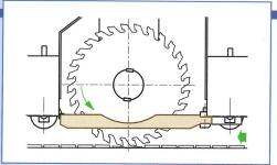
The long wooden shoe allows perfect holding of the plank, even if warped in the blade compartment, thus preventing the blades from removing or splitting cracked or thin planks.
