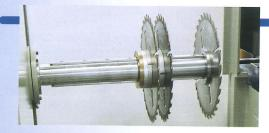
The surface treatment of the spindle ensures perfect running of the moving blade and long working life.
