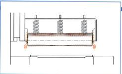
The rollers are guided at the side and they exert pressure over the entire width of the plank through three springs. This application also guarantees good holding of the planks which become curved after drying.
