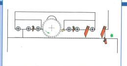
TOP ROLLERS GROUP raised automatically, with 6 independent hold-down rolls and a long wooden shoe placed between the blades. The splinterproof system consists of steel fingers distributed on 4 top rows (two of which acting as splinterproof and the other two as anti-kickback) and one bottom row.
