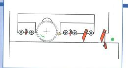
TOP ROLLERS GROUP raised automatically, with 5 independent hold-down rollers and a long wooden shoe placed between the blades.
